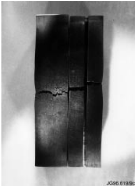
Figure 2. Sandia National Laboratory tests of JET belt limiter prototypes. After 4000 pulses at 4MW 2 , 1000 pulses at 4.5MW/m 2 . Electron beam irradiation.
