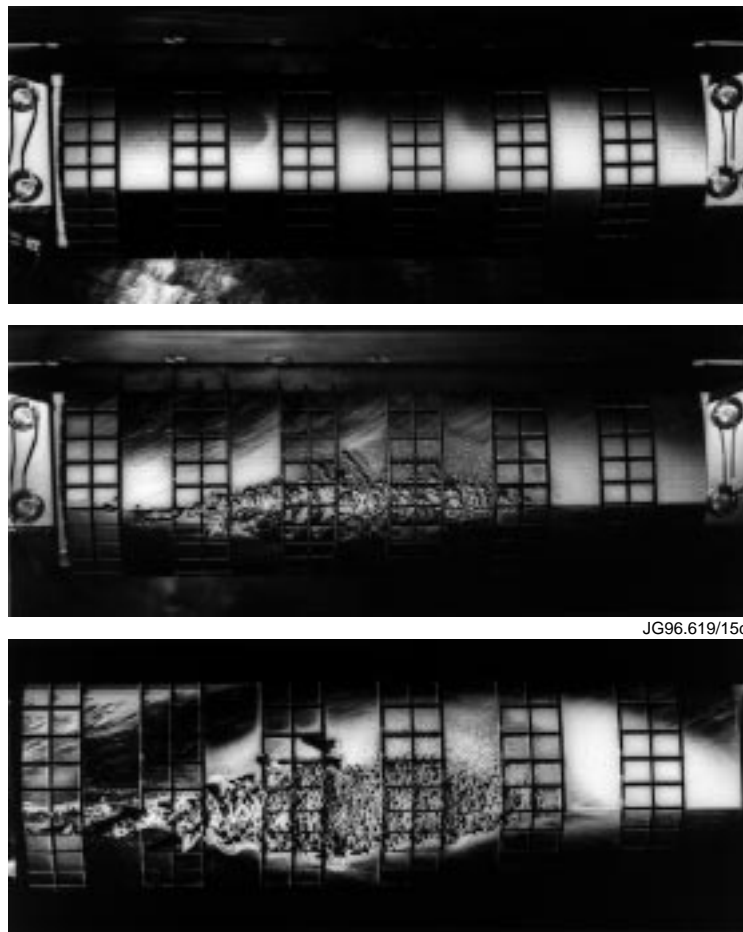
Figure 1. Three views of ISX-B Beryllium limiters. Note alternating castellated and uncastellated components. Top view, after initial ohmic operation, no melting evident. Middle view, after neutral beam heated discharges engendered some melting. Bottom view, after substantial edge melting with flux densities up to 40\text{MW/m}^2
