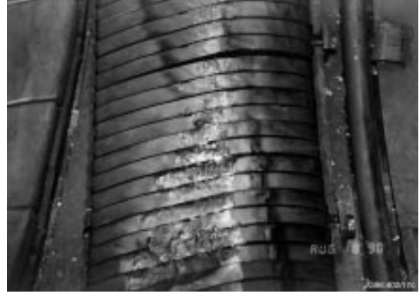
Figure 7. JET RF antennae tiles reused as target plates for X-point operation after plasma irradiation. Note significant material transport of molten material and no global cracking of the uncastellated tile. Initial edge flux densities up to 50\text{MW/m}^2 .
