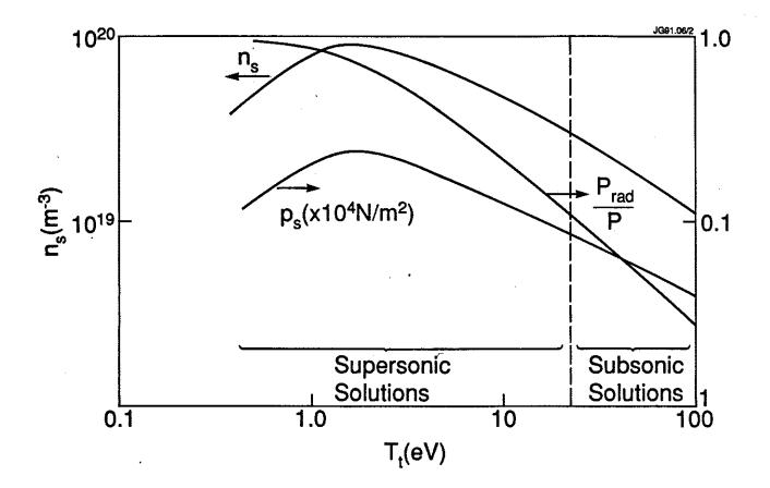
2. Upstream density n versus target temperature  $T_t$  resulting from different driving pressures  $p_s$ , for the specific case of P = 40 MW, L = 30 m, L<sub>i</sub> = 1 m, A = 0.4 m<sup>2</sup> and energy loss due to deuterium re-cycle (i.e., rather than fixed P<sub>r</sub>). Subsonic and supersonic solutions.
