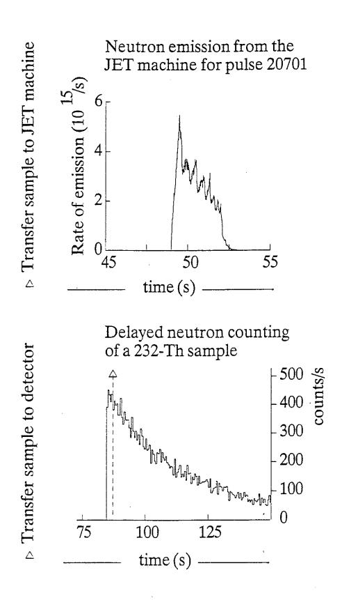
Fig 3. Illustrating the time sequence involved in the use of the delayed neutron counting system for a typical JET discharge.
