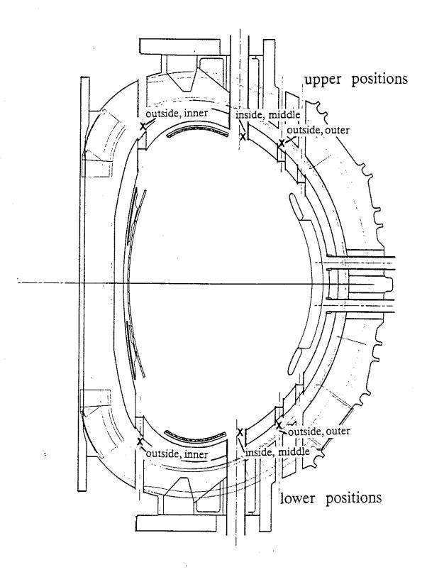
Fig 2. A drawing of a vertical section through the JET vacuum vessel, showing the location of the irradiation ends.
