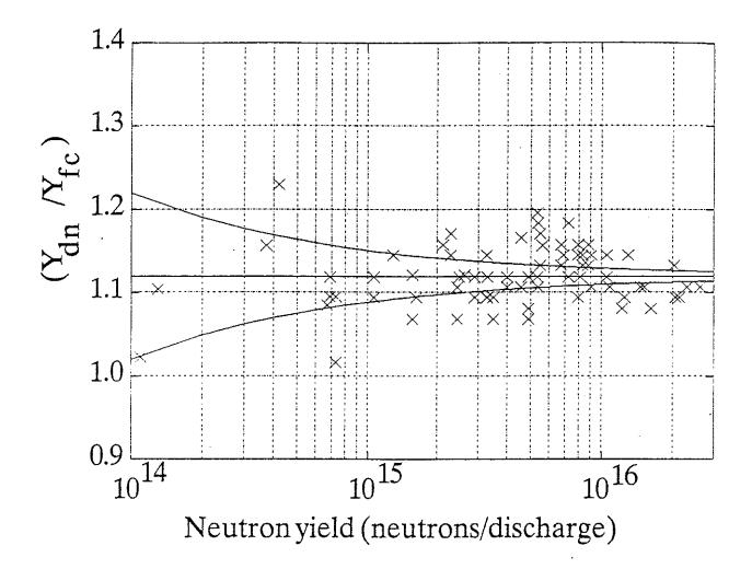
Fig 6. The ratio of delayed neutron/fission chamber neutron yields as a function of neutron emission strength. The solid curves indicate the  $\pm 2$  s.d. uncertainties attributable to counting statistics.
