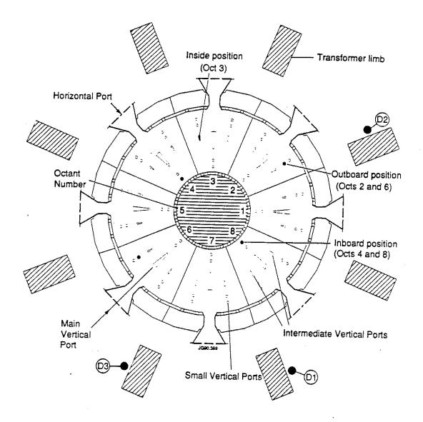
Fig 1. Section of JET at the horizontal mid plane, showing the positions of the fission chambers and of the irradiation ends.
