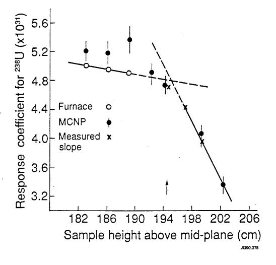
Fig 4. Showing the variation of the  $^{238}$ U response coefficient as a function of height above the tokamak horizontal midplane. The results of FURNACE and MCNP transport codes are compared and measurements of the gradient above the operating position are fitted to the MCNP data. The coefficient at 194.5 cm. is taken to be  $4.74 \times 10^{-31} \pm 5\%$ .
