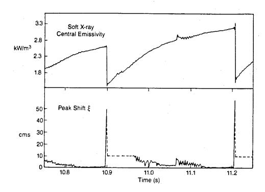
Figure 1. Showing the time behaviour of the displacement, ξ, of the peak soft X-ray emission, and its sudden increase at the time of the sawtooth collapse as indicated on the trace of the central soft X-ray emission. (The position of the peak emission is not well defined immediately following the collapse phase and is not therefore shown on the graph. The fluctuations which appear during the ramp phase have an m=1 structure but do not appear to directly influence the sawtooth behaviour).
