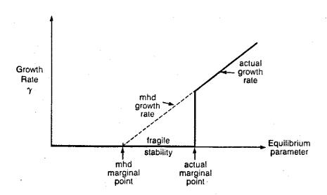
Figure 3. Illustrating a type of behaviour which would be consistent with the experimental observations. A weak stabilising effect provides a fragile stability beyond the mhd stability boundary. This allows the build up of free energy which is then suddenly released when the actual stability boundary is reached.
