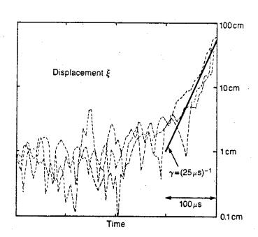
Figure 2. Graphs of the magnitude of the displacement, ξ, of the peak soft X-ray emission for three sawtooth collapses taken from different discharges. The initial noise level is ~lcm and the growth rises out of this noise with a growth rate of ~(25μs)<sup>-1</sup>, which increases the displacement to ~50cm in ~100μs. (The plasma current was 3.5MA, the toroidal magnetic field 2.9T and I.C.R.H. of 4-5MW was applied.)
