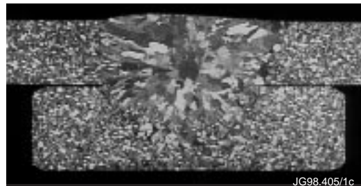
Fig 4 Macrograph section of completed orbital weld with insert ring
