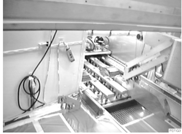
Figure 3. end effector remotely storing carriers into an ISO container
