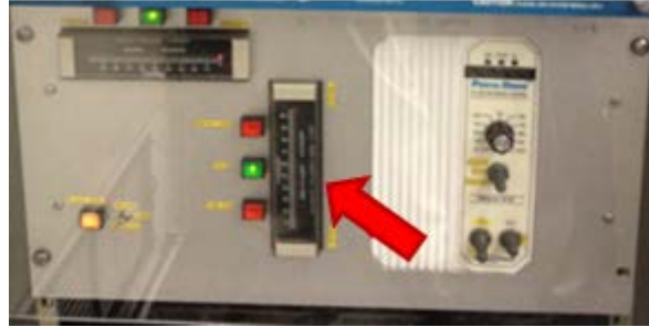
Figure 5.5. ^{241}\text{Am}/^9\text{Be} neutron source deployment device. The arrow indicates the position of the source in the horizontal camera, where the channel 4 is located.
