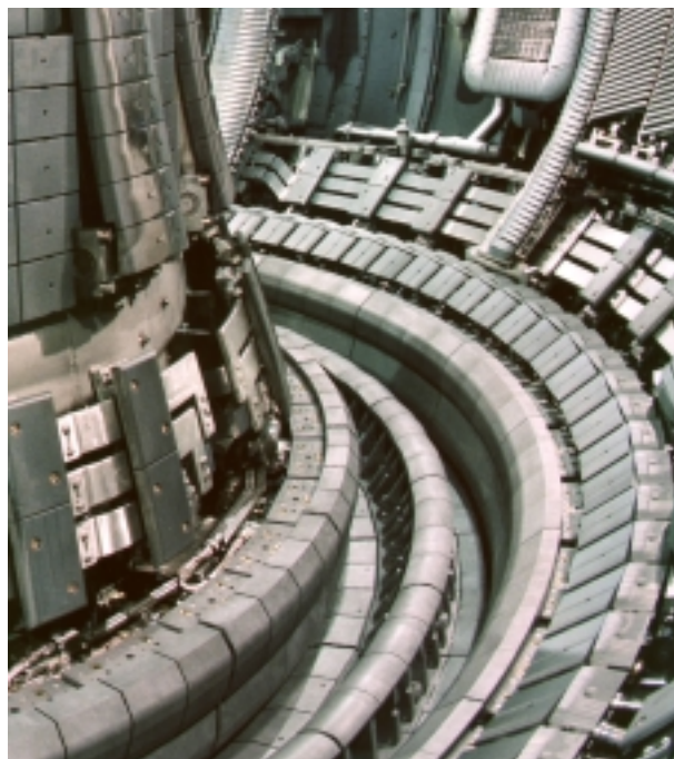
Figure 4.1: Shows an inside view of the torus with the Mark IIGB divertor used during the campaigns C1-C4
