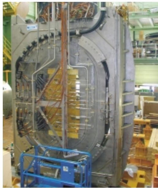
Figure 7.5: The Toroidal Field Model Coil ready for installation in the TOSKA test facility (Karlsruhe).
