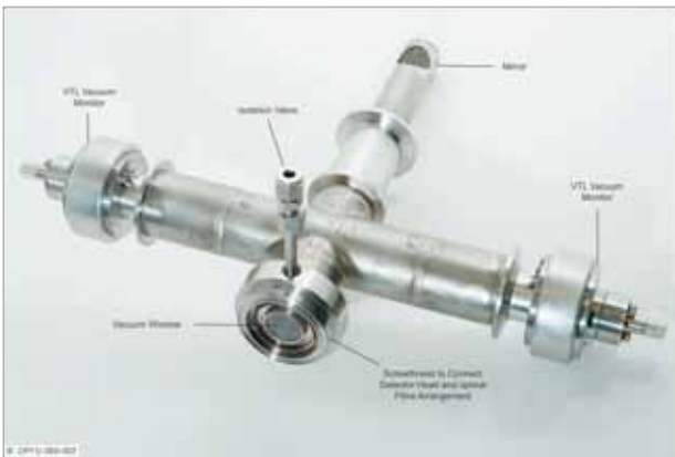
Figure 16: Spare detector showing the vacuum window, VTL pumping and mirror used in tests to assess why the installed VTL optical arc detection system failed.
