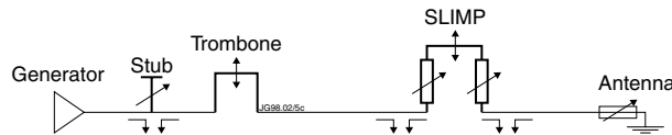
Figure 4: Schematic representation of the JET transmission lines including the Sliding Impedances (SLIMP).
