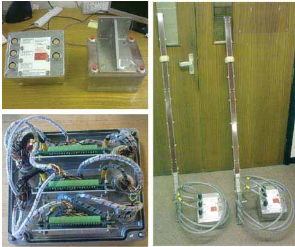
Figure 7: Assembly of the magnetic measuring instrumentation (housing, cables and probes support structure).
