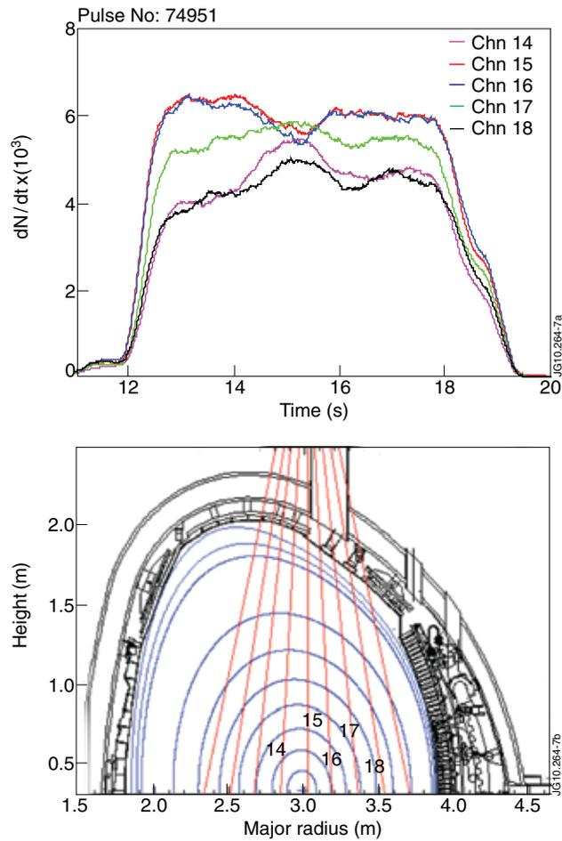
Figure 8: Top – 3.1MeV  $\gamma$ -ray intensities versus time recorded by vertical camera; bottom – the vertical camera lines of sight.
