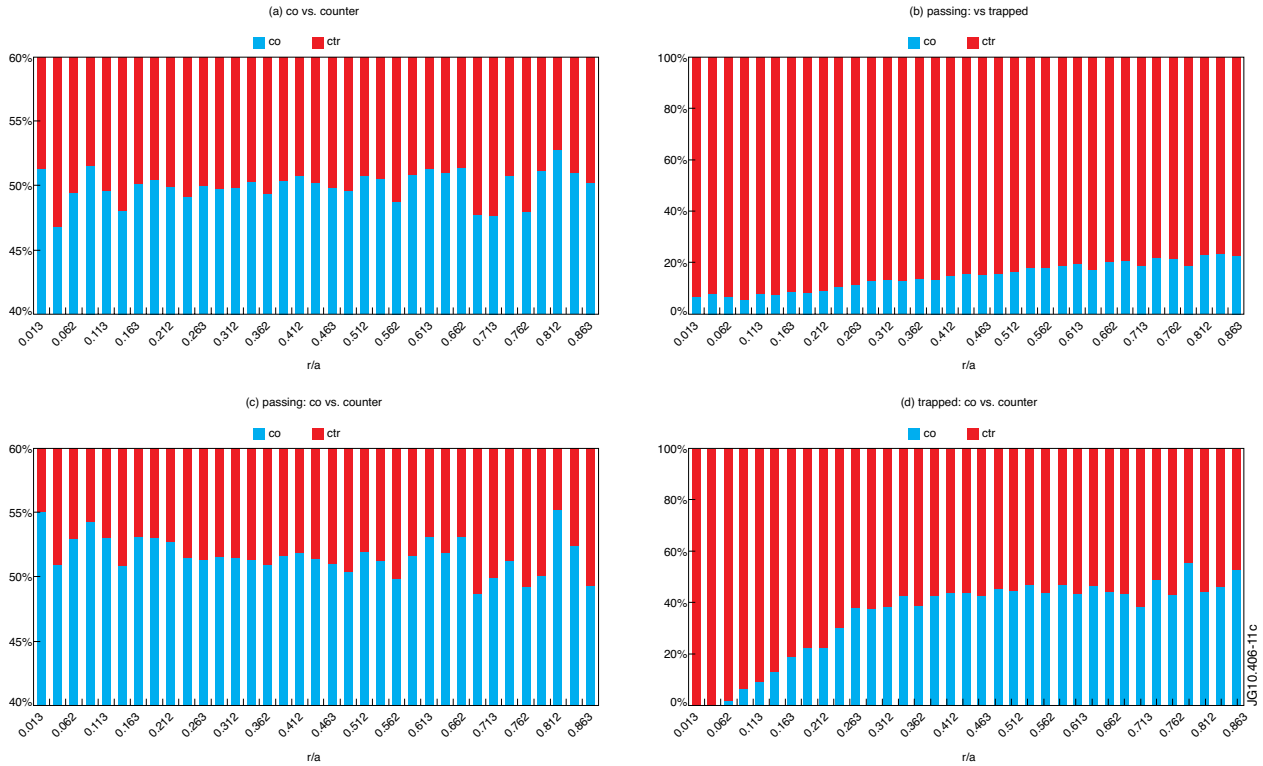
Figure A1. The ratio of co and counter test particles relative to (a) all particles, including both passing and trapped particles, (c) all passing particles and (d) all trapped particles in the W-RS configuration. (b) The ratio of passing and trapped test particles relative to all particles.
