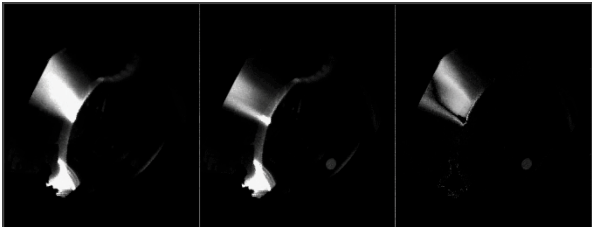
Two subsequent frames and their differences without vibrations but with a MARFE
