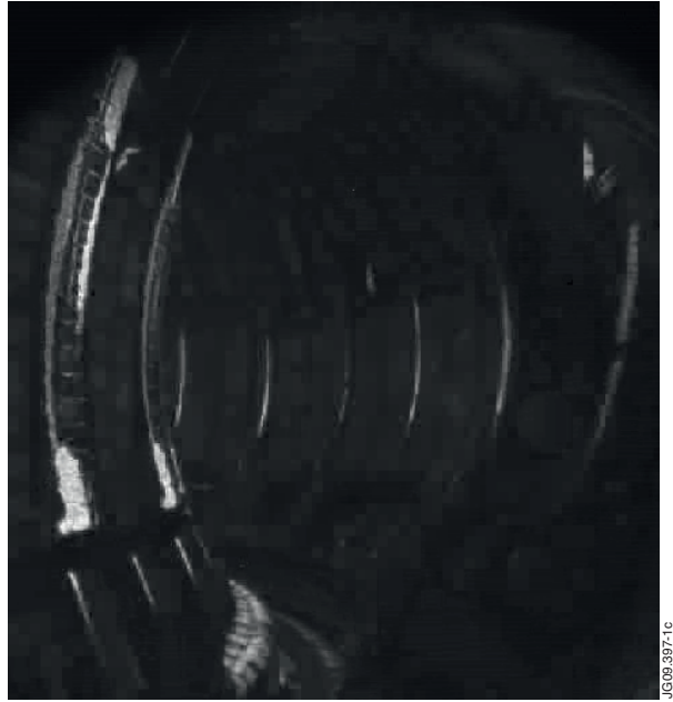
Figure 1: Example of image acquired by JET IR wide angle camera. The white pixels indicate regions of high surface temperature.
