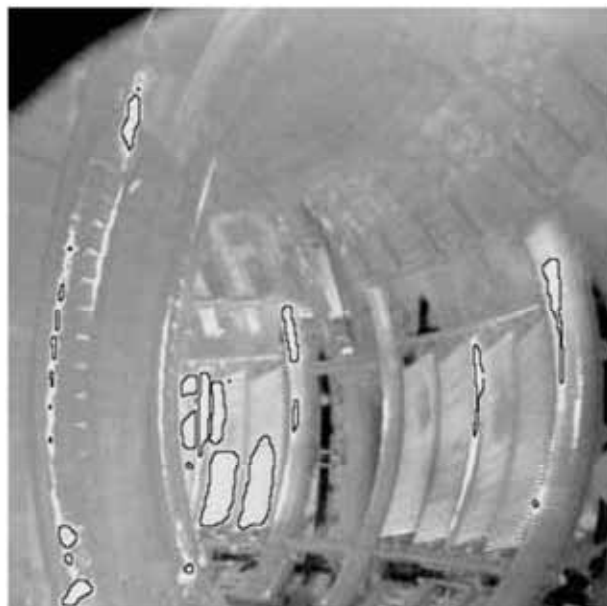
Figure 14: Example of static detection of hot spots. The contour of the detected regions is reported superimposed to the starting frame.
