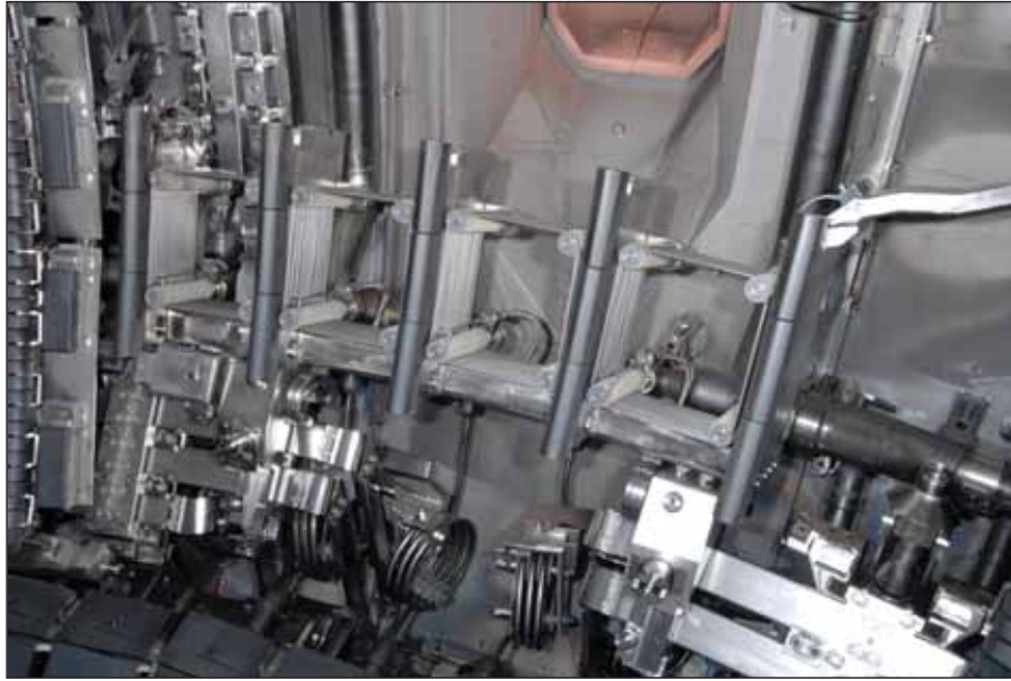
Figure 6: New JET intermediate- n antennas: front view of one group of four coils as installed in-vessel in October 2007. The second antenna frame is also installed in the toroidally opposite location at the same poloidal angle.
