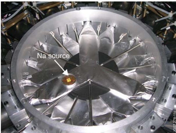
Figure 11: Photograph of the central S1 enclosure with ^{22}\text{Na} source ( T_{1/2}=2.605 years) in place on the top S1 detector layer. Also visible are the aluminum wrapped scintillator/light-guide assemblies with interposed black cardboard sheets besides light fiber guiding tubes.
