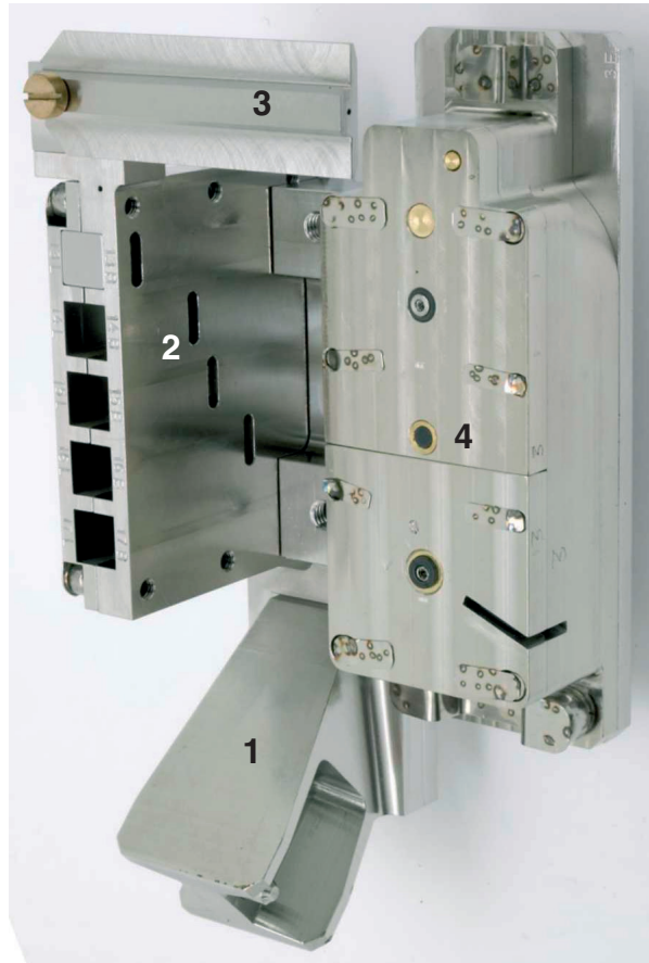
Figure 7: Bracket assembly for installation on the main chamber wall: holder (1); cassette with mirrors (2); magnetic shutter (3); rotatable deposition monitor (4).
