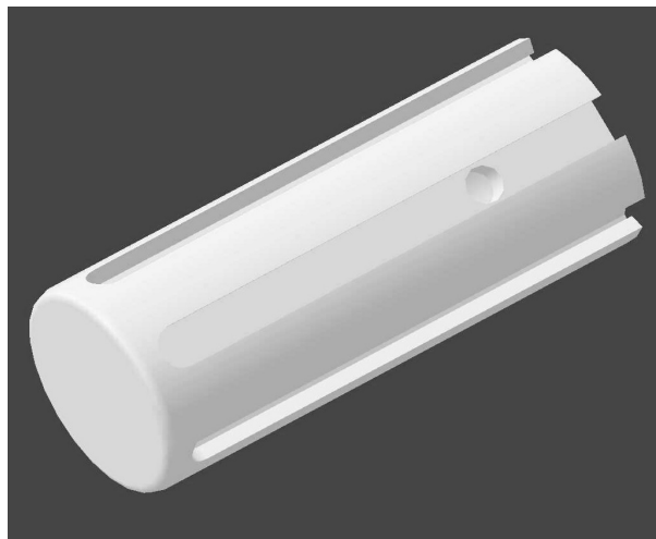
Figure 1: Sketch of the fast particle in-vessel activation probe: the six samples containing slots are regularly spaced and are 60 degree apart
