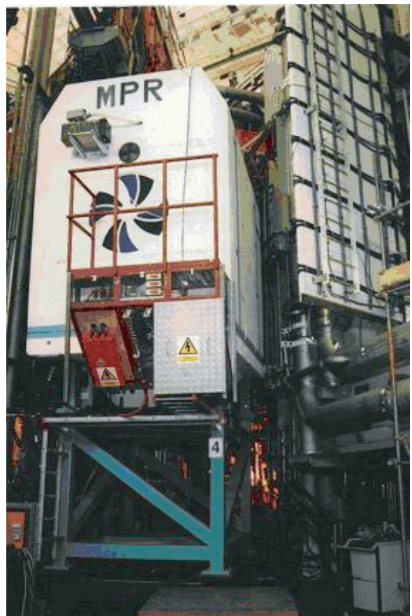
Figure 4: (a) The MPR neutron spectrometer (20 tons) under assembly of concrete blocks (66 tons) to protect the detector from extraneous background radiation. An extra local 2-ton lead shielding is enclosing the detector (bottom left). (b) The MPR installed in the Torus Hall. The overall size of the spectrometer is 1.9 \times 2.6 \times 0.8 \text{ m}^3 ( l \times h \times w ) that becomes 4.3 \times 3.9 \times 2.3 \text{ m}^3 including the shielding.
