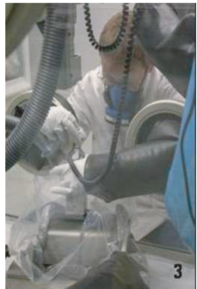
Figure 7: Handling facilities for beryllium and tritium contaminated materials in surface analysis laboratories: (a) loading samples to the analysis chamber in the accelerator laboratory at the University of Sussex; (b) coring of samples in the SIMS laboratory at VTT.
