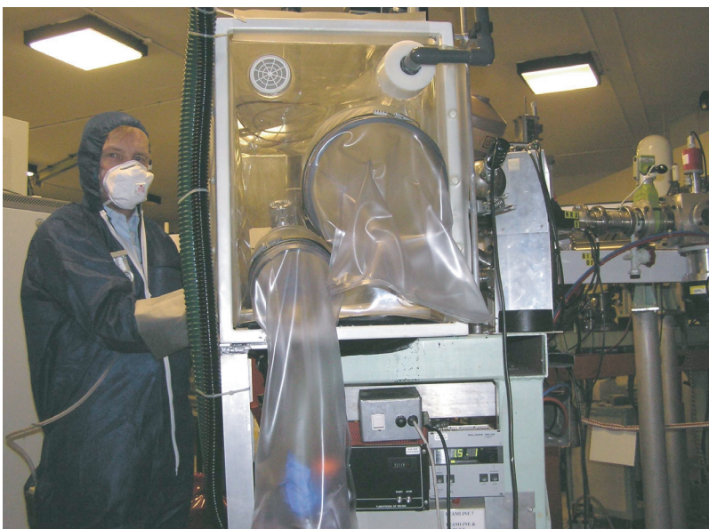
Figure 7: Handling facilities for beryllium and tritium contaminated materials in surface analysis laboratories: (a) loading samples to the analysis chamber in the accelerator laboratory at the University of Sussex; (b) coring of samples in the SIMS laboratory at VTT.
