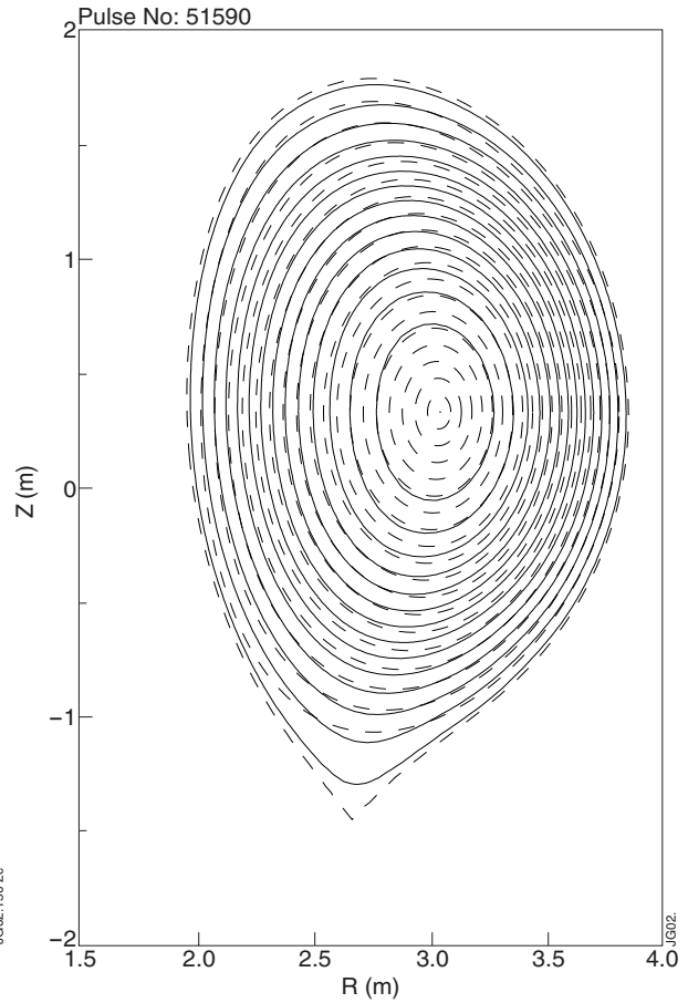
Figure.2: Comparison of EFIT magnetic topology with the one obtained by the described method.
