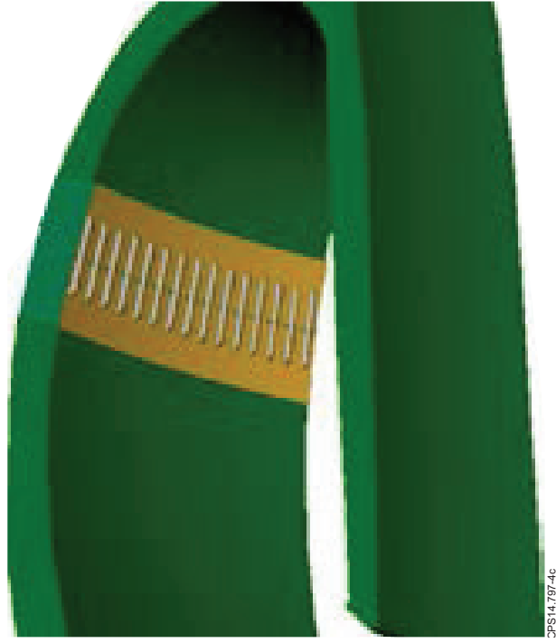
Figure 4. One sector of DEMO with an in-blanket IC antenna.
