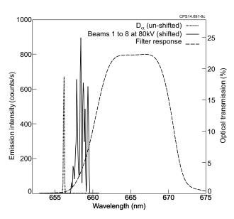
Figure 1: Calculated beam emission for 80kV deuterium beams. The Doppler shifted emission from full, half, and one third energy components is plotted. The transmission of the angle tuned (15°) interference filter is included.
