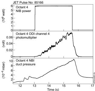
Figure 2: Doppler shifted Da emission measured from the neutral beams duct with constant beam power and increasing duct pressure [JET Pulse Number: 85166].
