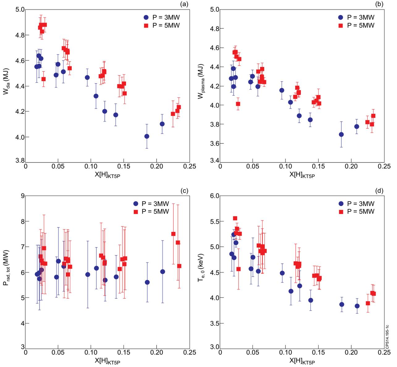
Figure 2: Diamagnetic energy (a), plasma stored energy (b), total radiated power, (c) and ECE central electron temperature (d) as a function of the minority concentration evaluated spectroscopically in the edge from the ratio of line intensities  $H_{\alpha}/D_{\alpha}$  (KT5P diagnostic).
