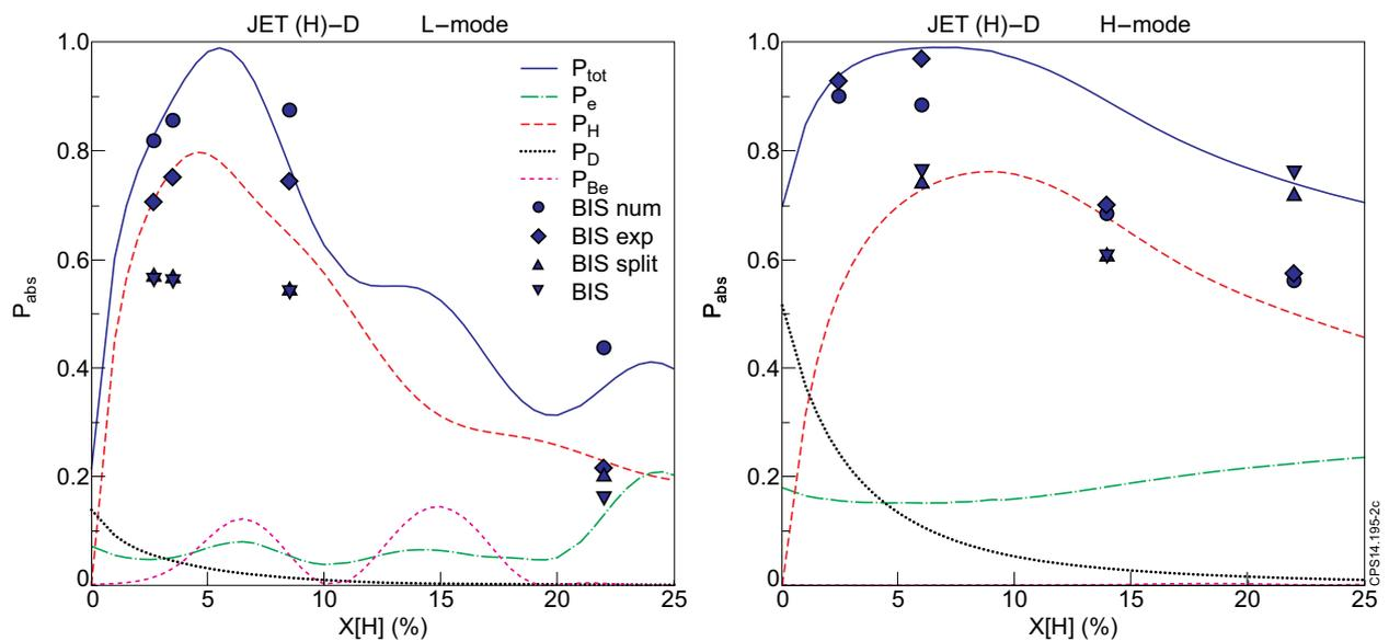
Figure 1: Heating efficiency in L-mode (left) and H-mode (right) as a function of the minority concentration. The symbols represent the experimental data inferred from BIS analysis; the lines are the corresponding theoretical predictions for the absorption in a full transit over the plasma.
