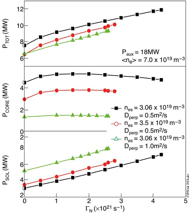
Figure 4: Plasma parameters versus nitrogen puff level for different edge densities,  $n_{es} = 3.06 \times 10^{19} \text{ m}^{-3}$ ,  $n_{es} = 3.5 \times 10^{19} \text{ m}^{-3}$  and different radial diffusion coefficients in the SOL,  $D_{\perp} = 0.5 \text{ m/s}$ ,  $D_{\perp} = 1 \text{ m/s}$ : a) total radiation losses, b) core radiation, c) SOL radiation.
