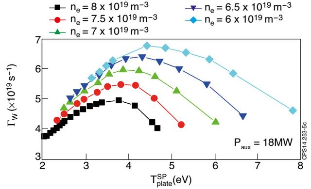
Figure 5: Tungsten flux versus electron temperature at the strike point for auxiliary heating power  $P_{aux} = 18 \text{ MW}$  and different plasma densities  $\langle n_e \rangle = 6 \div 8 \times 10^{19} \text{ m}^{-3}$ .
