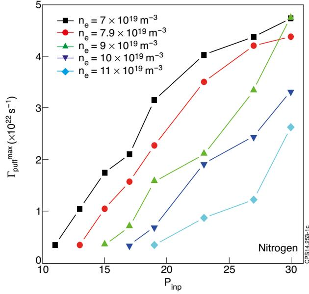
Figure 1: Maximum allowed nitrogen puff level for JET ILW discharges.
