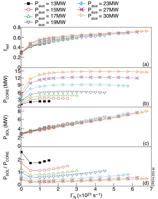
Figure 3: Plasma parameters versus nitrogen puff level for plasma density  $\langle n_e \rangle = 7 \times 10^{19} \text{ m}^{-3}$  and auxiliary heating powers  $P_{\text{aux}} = 13 \div 30 \text{ MW}$ : a) radiation fraction, b) core radiation, c) SOL radiation and d) ratio between SOL and core radiations.
