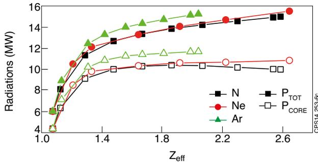
Figure 6. Total radiation losses ( $P_{TOT}$ ) (full symbols) and core radiation ( $P_{CORE}$ ) (open symbols) for different seeding gasses:  $N_2$ ,  $Ne$ , and  $Ar$ .
