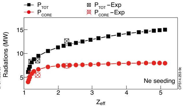
Figure 9. Calculated total radiation losses ( $P_{\text{TOT}}$ ) (squares) and core radiation ( $P_{\text{CORE}}$ ) (circles) versus  $Z_{\text{eff}}$  value for neon seeding together with experimental points for JET shots: 85438, 85439, 85441.
