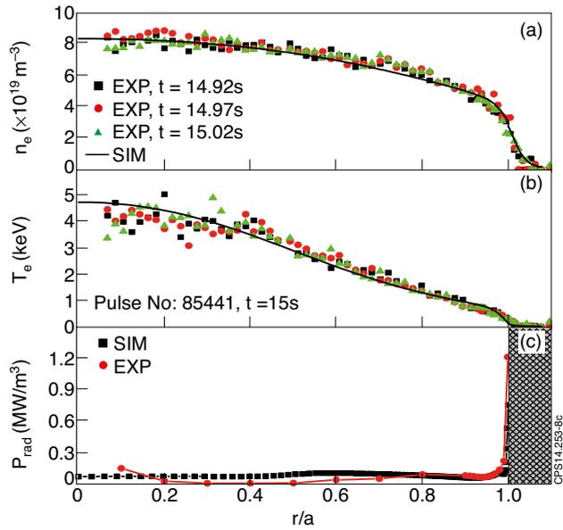
Figure 8. Experimental electron density (a) and electron temperature (b) profiles from HRTS diagnostic at different times and from COREDIV simulations, as function of the normalized minor radius for the JET shot 85441. For the same shot radiation profiles in the core from experiment and from simulations (c).
