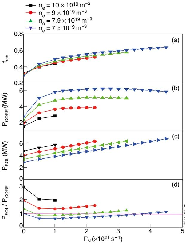
Figure 2: Plasma parameters versus nitrogen puff level for auxiliary heating power  $P_{\text{aux}} = 19 \text{ MW}$  and different plasma densities  $\langle n_e \rangle = 7 \div 10 \times 10^{19} \text{ m}^{-3}$ : a) radiation fraction, b) core radiation, c) SOL radiation and d) ratio between SOL and core radiations.
