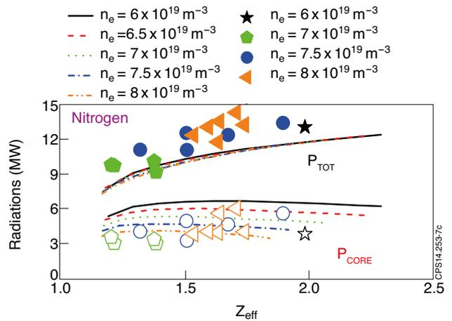
Figure 7. Experimental (points) and simulated (lines) values of total radiation losses ( $P_{TOT}$ ) (full symbols) and core radiation ( $P_{CORE}$ ) (open symbols) versus  $Z_{eff}$  value for different plasma densities and nitrogen seeding levels ( $Z_{eff}$  is almost linear function of the nitrogen influx).
