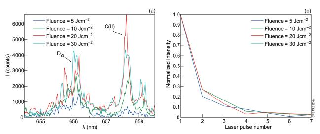
Figure 2: a) The signal-to-noise ratio of the  $D_{\alpha}$  line increases with fluence, b) The shape of the depth profile of D remains constant with increasing fluence.
