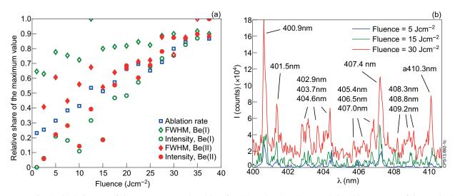
Figure 1: a) The behavior of the intensities and widths of Be(I) and Be(II) lines and the ablation rate of the studied coating as a function of the laser fluence, b) W(I) lines measured with different fluences, showing the increasing quasi background due to the weak W(I) lines around the most intense lines at 400.9nm, 407.4nm, and 410.3nm.
