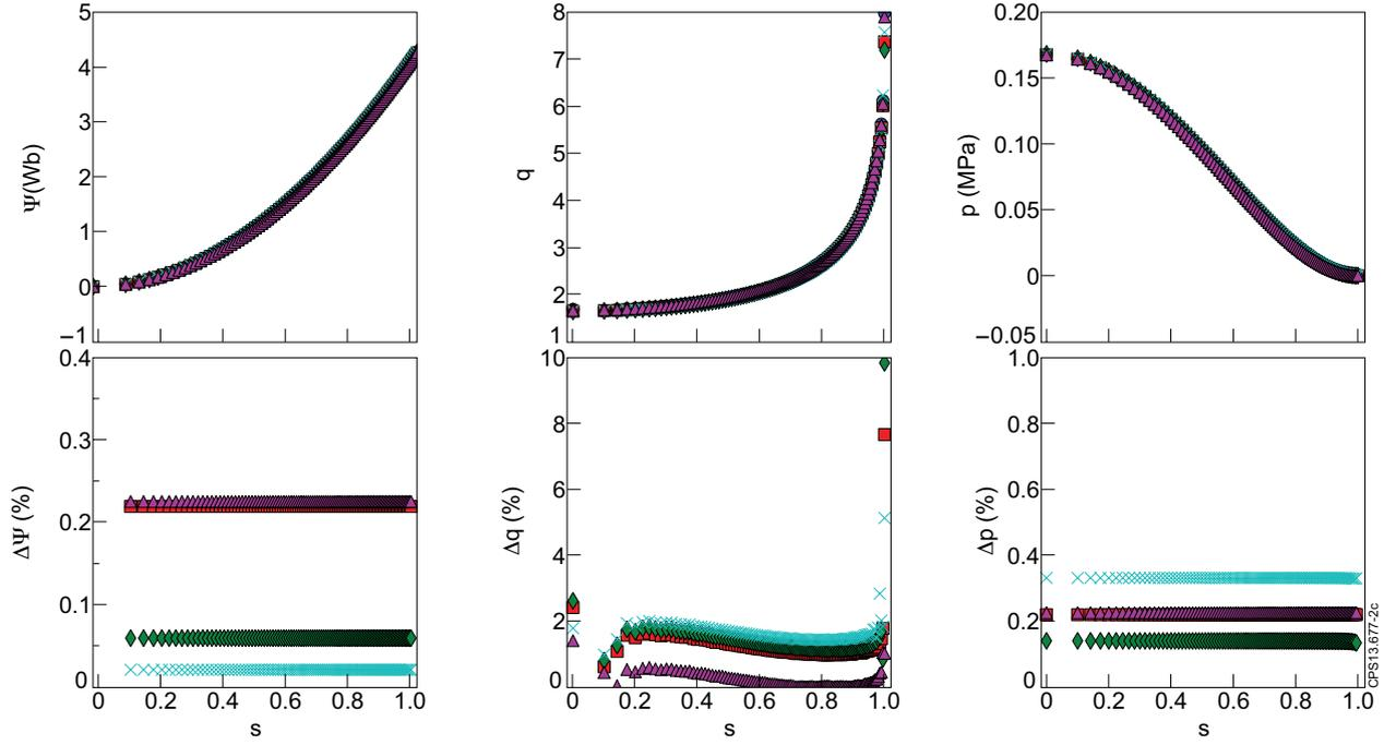
Figure 2: Comparison of the profiles and correspondent accuracies of the poloidal flux (a,d), safety factor (b,e), pressure (c,f). Blue(circles)-EQUAL, red(squares)-CHEASE, green(diamonds)-SPIDER, cyan( $\times$ )-HELENA, magenta(triangles)-CAXE.
