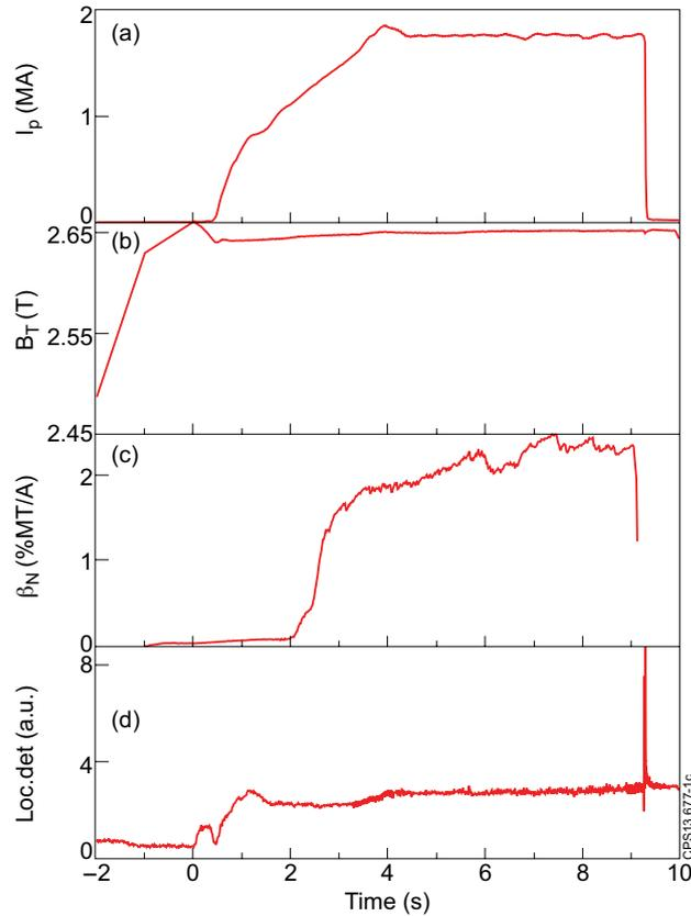
Figure 1: Time traces of plasma parameters for the JET Pulse No: 74221. a) plasma current; b) toroidal magnetic field; c) normalized beta; d) locked mode amplitude
