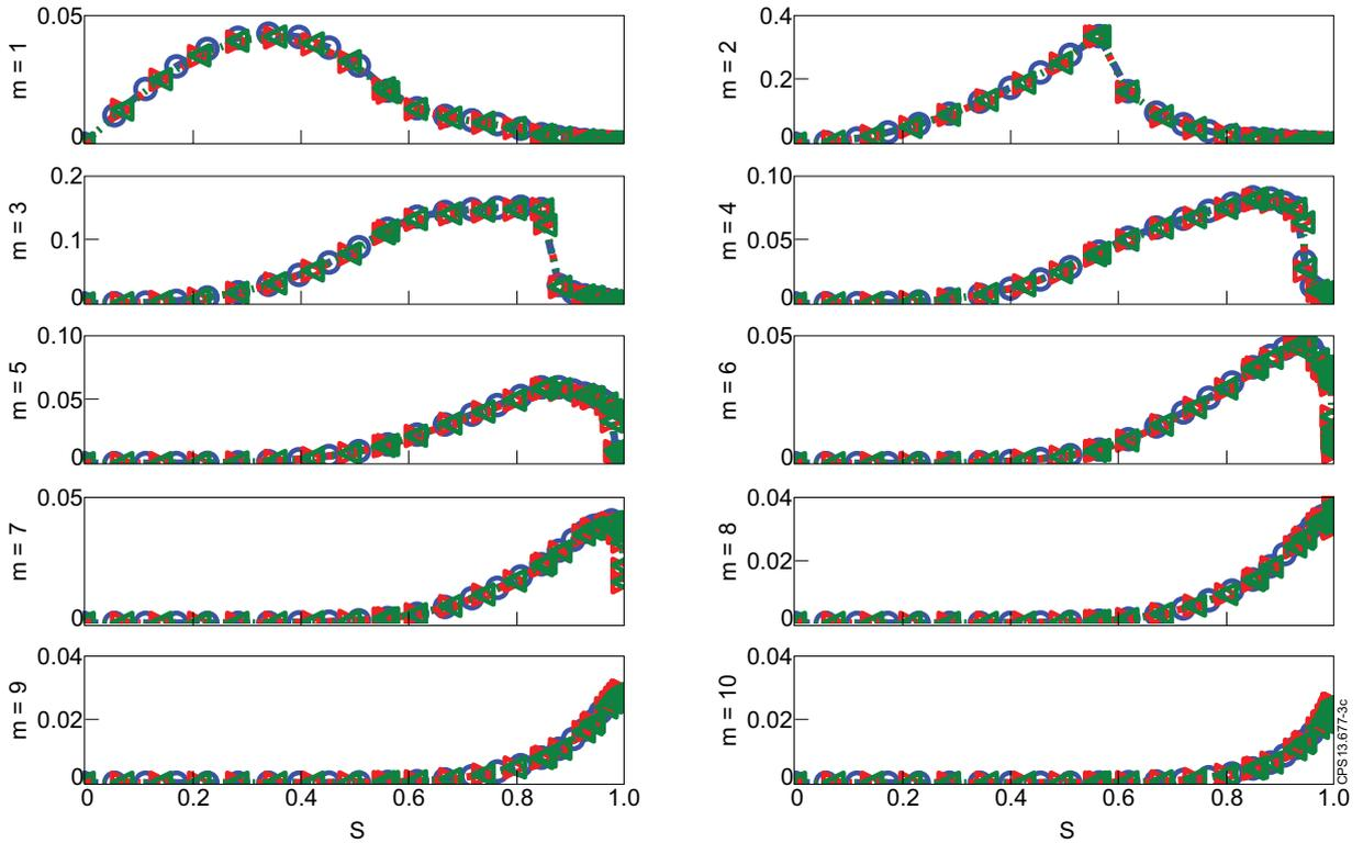
Figure 3: Poloidal Fourier components ( $m = 1-10$ ) of the normal displacement  $\xi_n$ . Blue – KINX, red – MARS-F, green – MARS.
