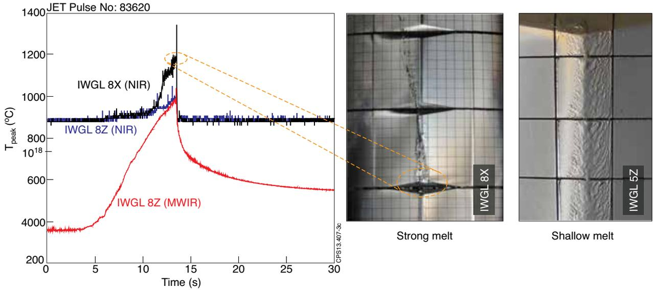
Figure 3: (a) Peak temperature,  $T_{peak}$  measured on the IWGL 8Z by the MWIR camera (red) and by the PIW (NIR, 1m) camera (blue), and on the IWGL 8X by the PIW camera (black). (b) Picture of the melt damage that occurred during JET Pulse No: 83620 on the IWGL 8X. The melt damage coincides with the plasma contact point.
