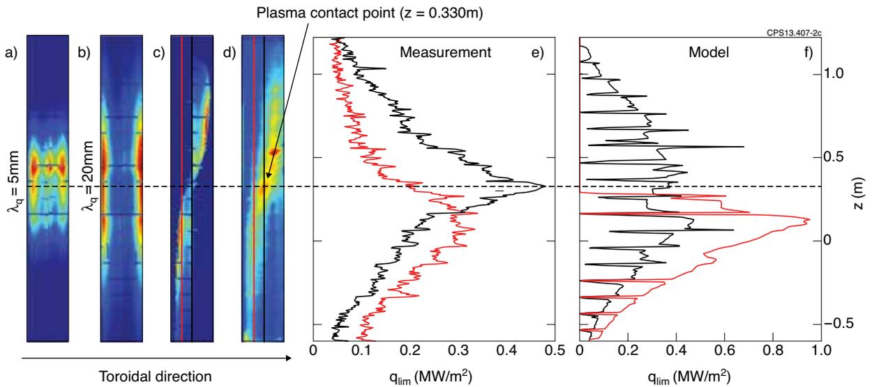
Figure 2: Heat flux map on the IWGL predicted with PFCFLUX (a) without and (b) with shadowing. (c) heat flux map derived from IR thermography. (d) and (e)  $q_{lim}$  poloidal profiles at the centre ( $\phi = 1:06$ ) and on the left wing ( $\phi = 1:04$ ) from the map (b) and (c) respectively.
