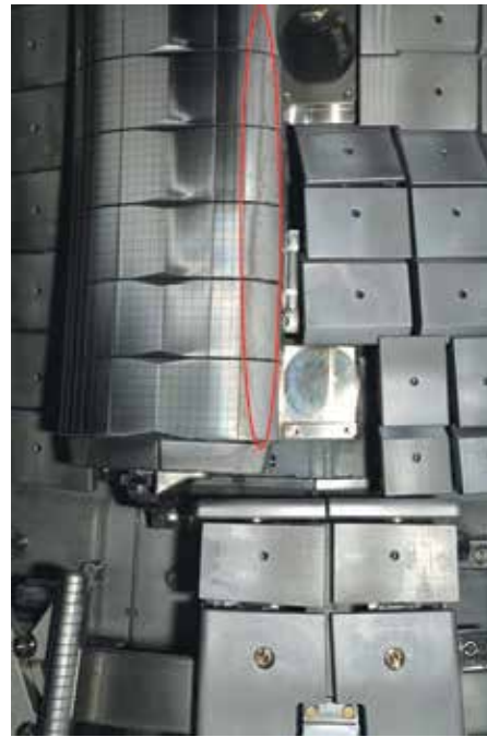
Figure 3: Deposits of Be on W-coated wings, inner wall, bottom of limiter beam, Octant 7.
