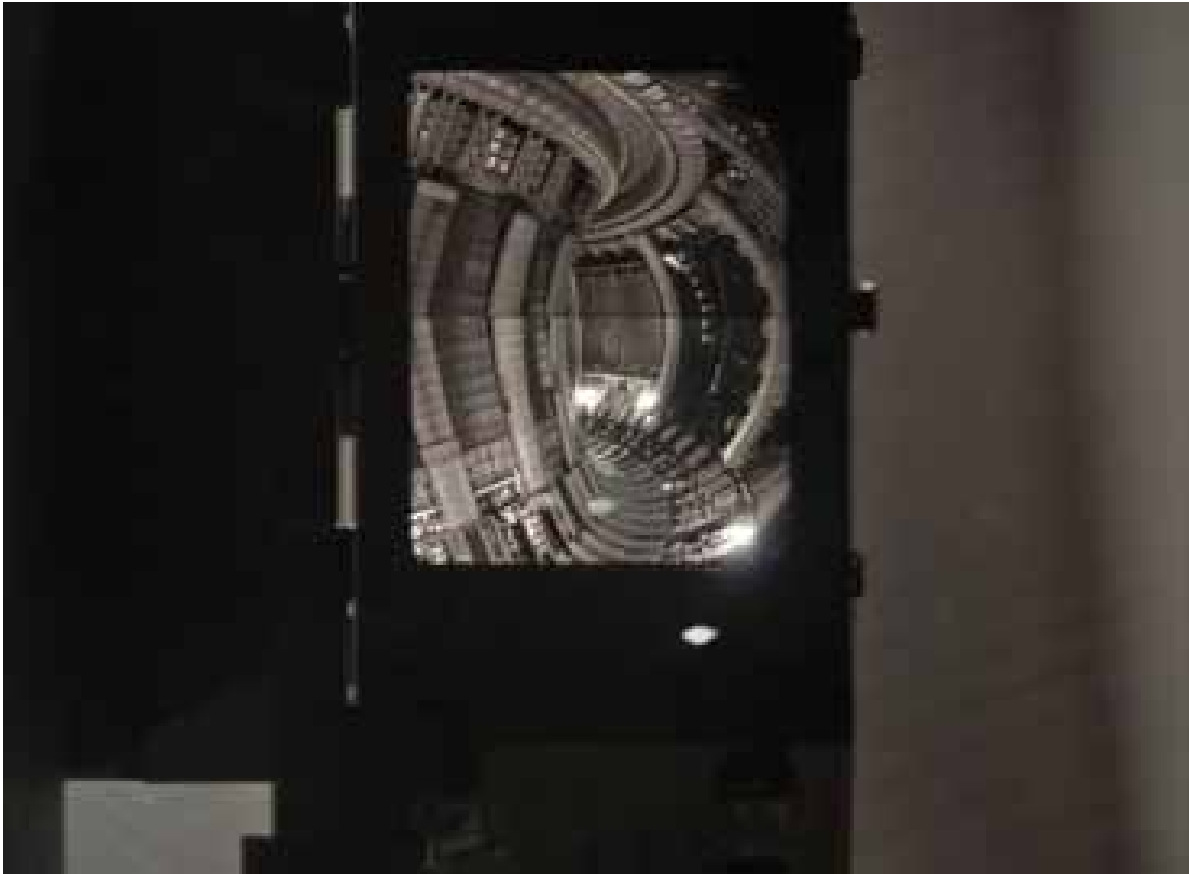
Figure 1: In-vessel mirror box with intermediate image showing a wide angle view of the inside of the JET vacuum vessel (upside down).
