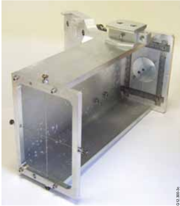
Figure 3: Alignment bracket prior to installation. The convex mirror in the rear plate was used to determine corrections to the horizontal and vertical tilt. The cross wires in the front plate together with markings on the rear plate provided a second independent measurement.
