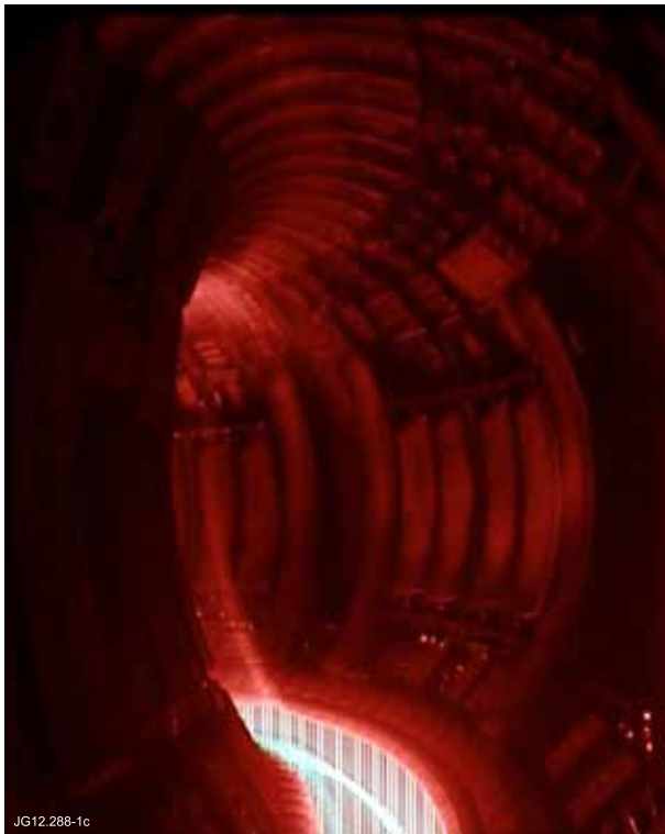
Figure 1. A frame of the operation visible camera KL1. A halo of increased emission, which is believed to indicate the position of the plasma boundary is clearly visible. (Pulse No: 82080)
