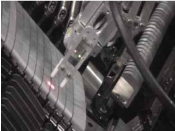
Figure 4: Inspection of the installed Lower Hybrid frame.
