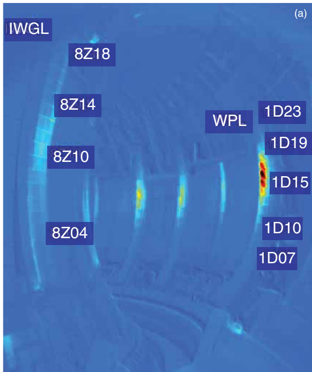
Figure 2a: Image taken with the wide angle view IR camera (KL7). The tile names on the inner wall guard limiter 8Z and the outer poloidal limiter 1D indicate the tiles fitted with thermocouples. Figure 2b: Temperature increase observed for a similar pulse. The TC C shows a greater increase due to its proximity to the plasma contact point. Thermalisation within tiles occurs after 500 sec. Figure 2c shows that the agreement between surface temperature measured by IR and protection cameras are within 100°C.
