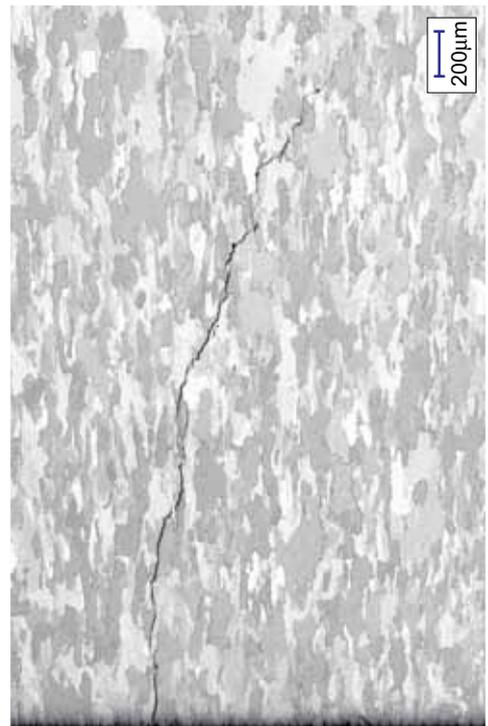
Figure 6: Crack found at the upper edge of the racetrack hole.
