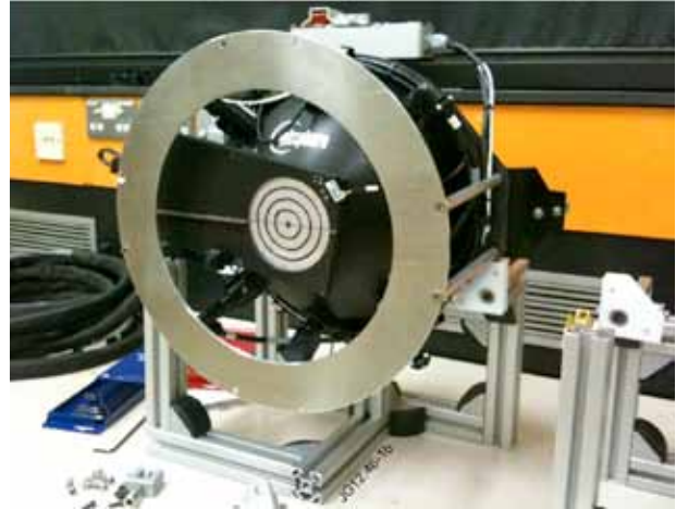
Figure 1: (a) CAD drawing of the ICLS head, and (b) photograph of as-built ICLS, resting in the transport cradle.
