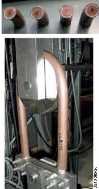
Figure 2: Above: Sections Cut from the U bend test, Below the U-Bend test fixture.
