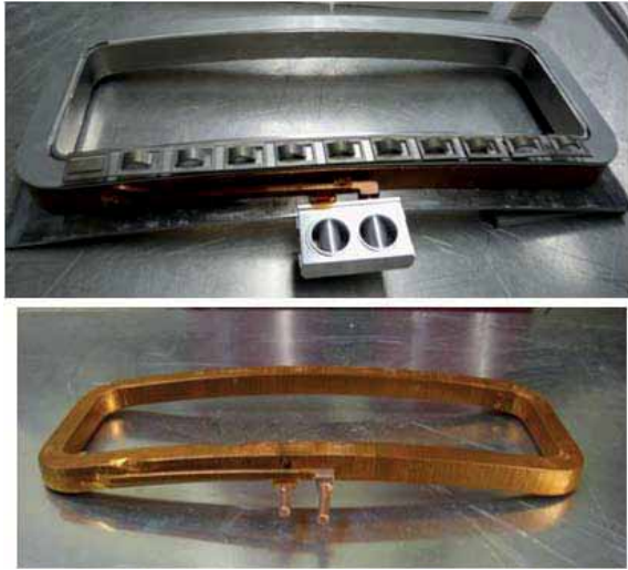
Figure 10: DIII-D CP Coil Components. At Left: Coil cover and one of the four strips of Inconel 718 springs, the Bonded Coil At Right, the Preload Assembly Fixture.
