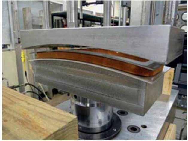
Figure 10: DIII-D CP Coil Components. At Left: Coil cover and one of the four strips of Inconel 718 springs, the Bonded Coil At Right, the Preload Assembly Fixture.
