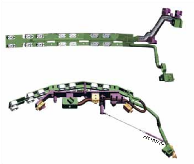
Figure 2: View of a Dump Plate Thermocouple and Halo Coil Conduit /Loom and RH Tool designed for the JET Torus.
