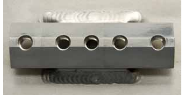
Figure 3: Diagnostic JET Torus Welded Rail.
