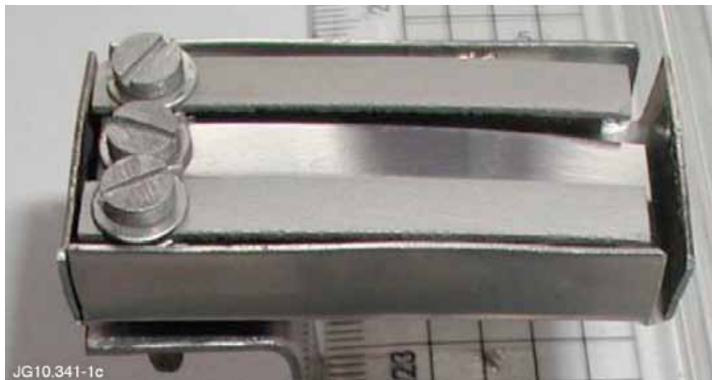
Figure 1: Experimental device for investigation of the global stress.
