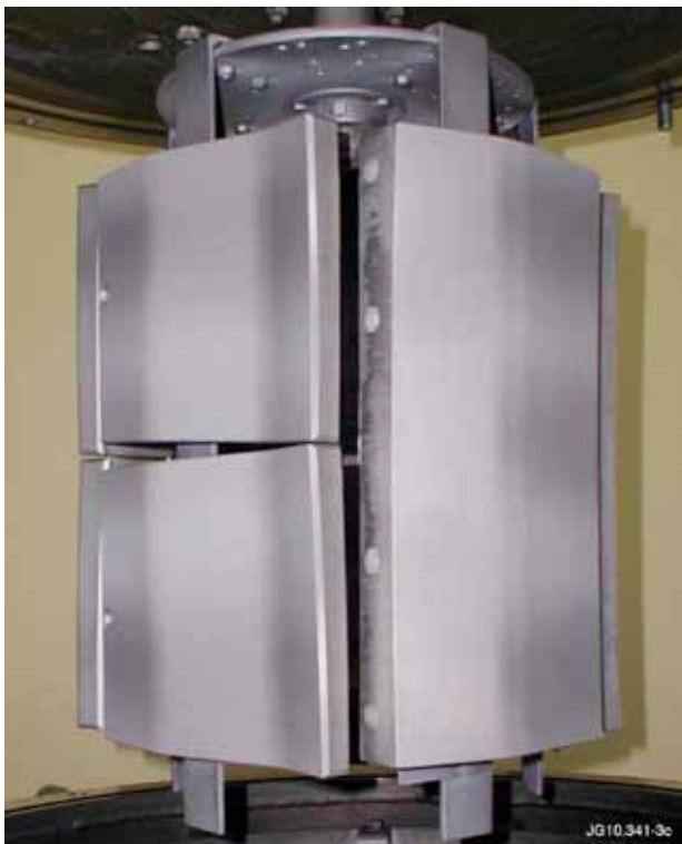
Figure 3: G6 and G7 divertor tiles coated with 20-25 μm W in series production.
