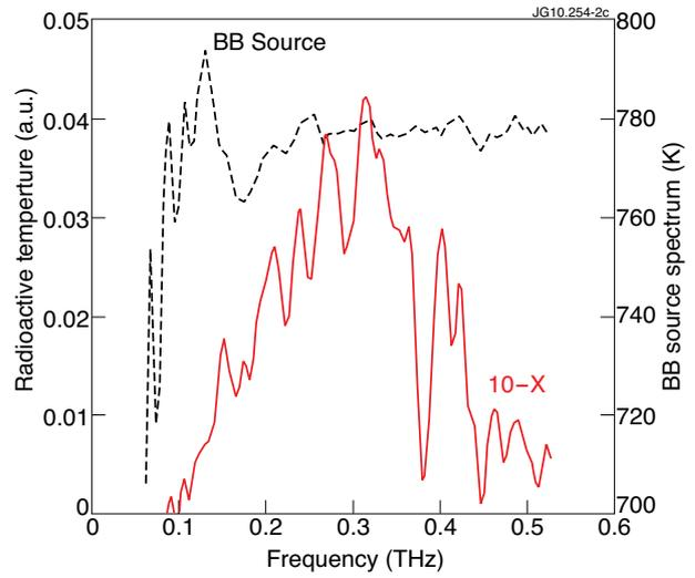
Figure 3: Spectra of hot BB source: nominal (dashed) and measured with 10-X (solid) channel.
