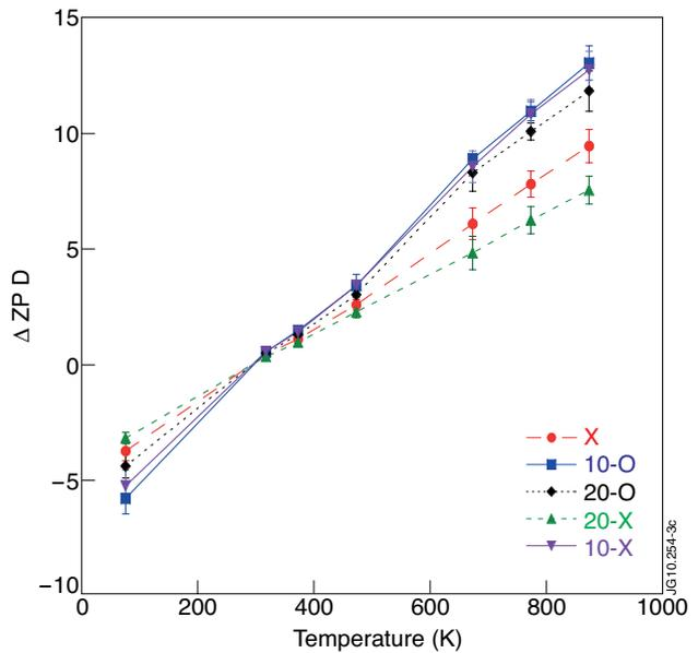
Figure 5: ZPD (peak-to-valley) amplitude versus BB temperature (ex-Vessel measurements). The slope is as defined in (1).
