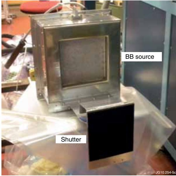
Figure 2: Hot blackbody source built by CCFE, used in the Vessel.
