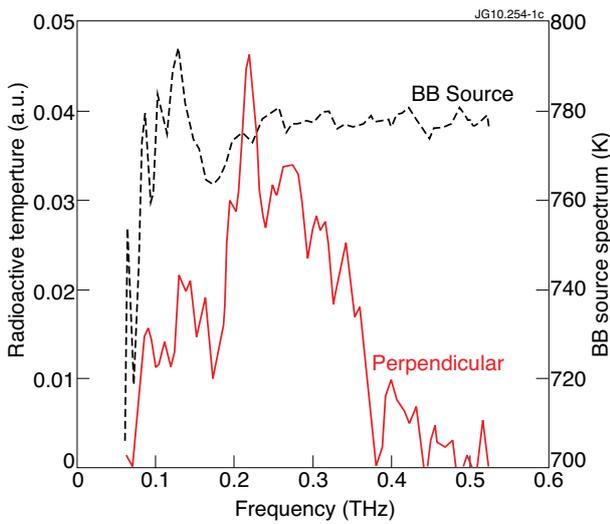
Figure 4: Spectra of hot BB source: nominal (dashed) and measured with perpendicular channel (solid).
