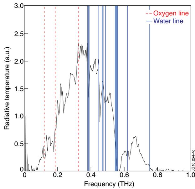
Figure 1: Spectra of hot BB source measured with perpendicular channel. A few water and oxygen lines are shown.
