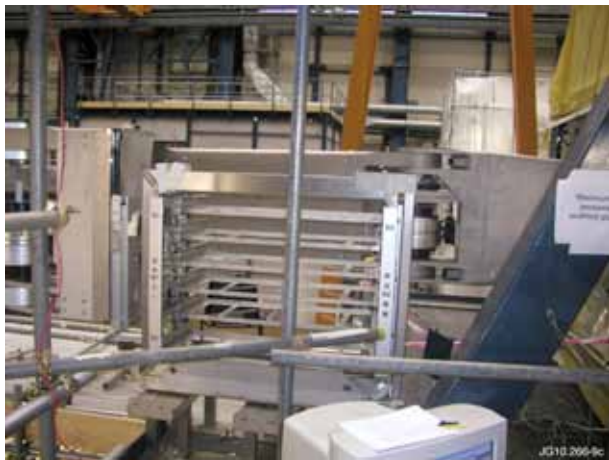
Figure 9: Sequence of photo's The Extended Octant 1 boom using the vertical traverse system to collect a task module during commissioning in 2009.
