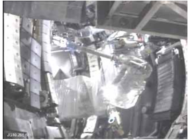
Figure 6: Photograph of the manipulator and task module at work in the EPII shutdown. The manipulator is installing inconel inner wall guard limiter tiles to the beam on the left of the photograph, and the task module is at the top of the photograph, with tiles loaded for installation.
