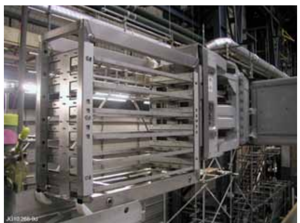
Figure 9: Sequence of photo's The Extended Octant 1 boom using the vertical traverse system to collect a task module during commissioning in 2009.
