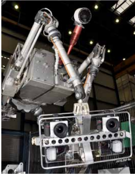
Figure 4: Stereophotogrammetry camera held by Mascot
