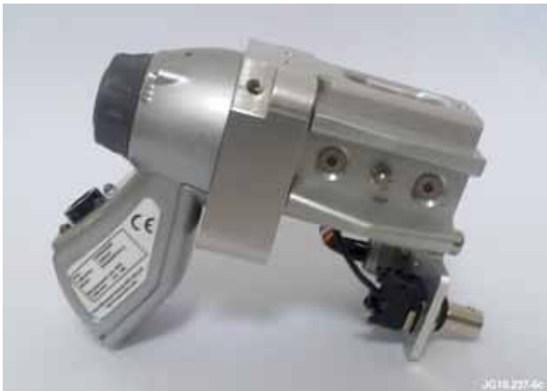
Figure 6: RH compatible GapGun sensor
