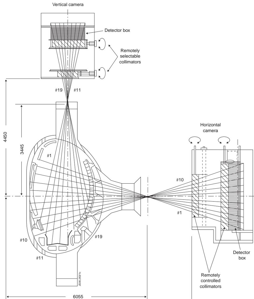
Figure 4: The topology of the neutron camera lines of sight.
