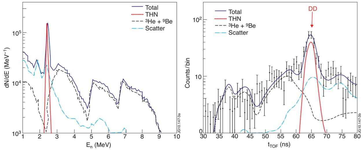
Figure 3: Various components of the neutron spectrum, versus time of flight (top) and energy (bottom).
