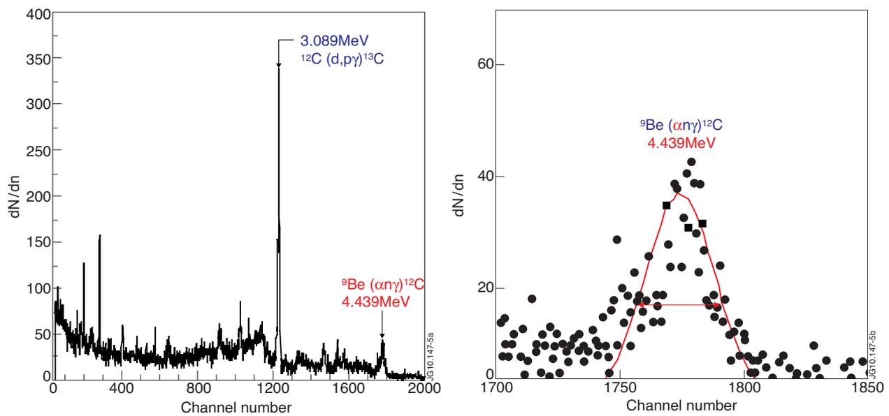
Figure 6: Top: the spectrum measured with a HPGGe detector, showing various emitted lines with unprecedented energy resolution. Bottom: the doppler broadening of the 4.439 MeV line, corresponding to a temperature of about 200 keV
