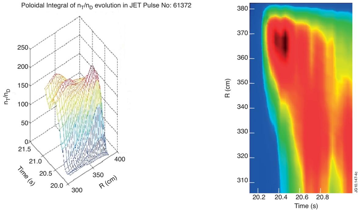
Figure 5: Time evolution of the tritium content after gas puffing in an experiment of the 2003 Trace Tritium campaign in JET.
