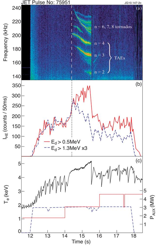
Figure 2: Top: signature of the TAE modes in the frequency spectra of the magnetic pick-up coils. Middle: evolution of the neutron emission due to deuterons in the energy intervals above 0.5MeV (red continuous line) and above 1.3MeV (blue dashed line) Bottom: electron temperature of the plasma and the additional heating powers: blue dashed line ICRH, red continuous line NBI.
