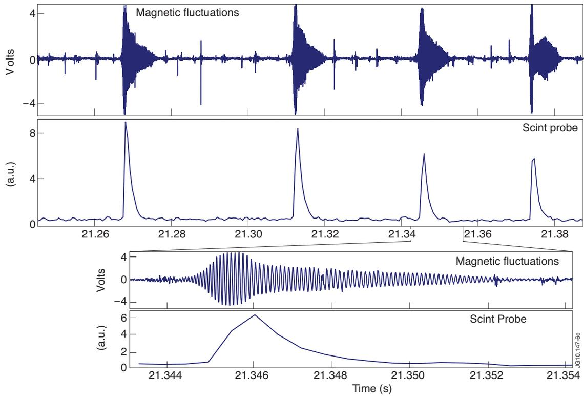
Figure 7: Magnetic fluctuation time trace with four fishbones, together with one of the photomultiplier signals of the scintillator diagnostic. Below expanded view for a single fishbone. After the maximum is reached, the fast ion loss is limited by the finite decay time of the scintillator material.
