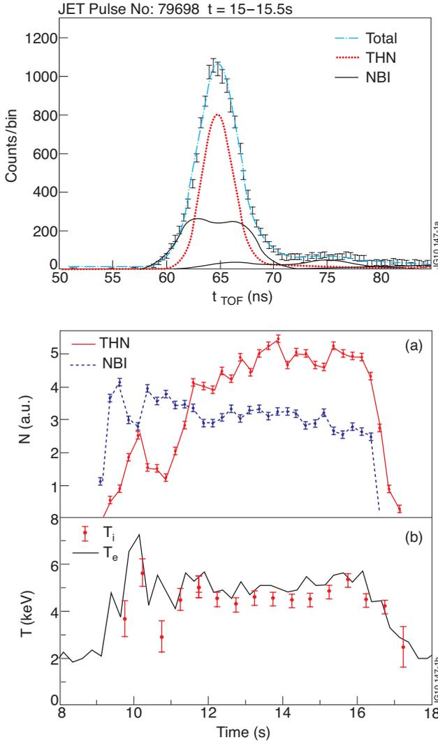
Figure 1: Top- the neutron (TOF) spectrum measured by TOFOR for a 4.5MA, 3.6 T discharge. Almost 70% of the emission is thermal (THN) in the high heating phase of the discharge and the rest is due to the beam plasma interaction (NBI) Middle: the time evolution of the neutron emission shows that the thermal dominated period lasts for about 4 seconds. Bottom: the estimate of the ion temperature from TOFOR compared with the electron temperature determined with Thomson Scattering.
