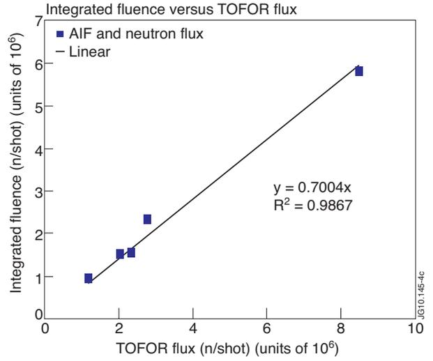
Figure 4: Area Integrated Fluence (AIF) versus the TOFOR flux.
