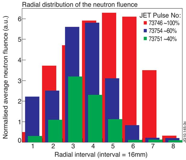
Figure 3: Radial distribution of the neutron fluence for three different pre-collimator openings.
