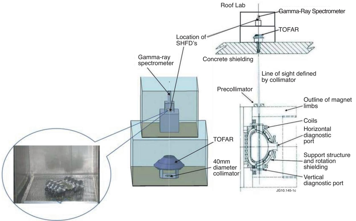
Figure 1: Experimental setup for SHFD neutron measurements along the JET KM11 Line-of-Sight. (insert) Bubble detectors (SHFD's) set installed on the KM11 neutron beam line-of-sight.
