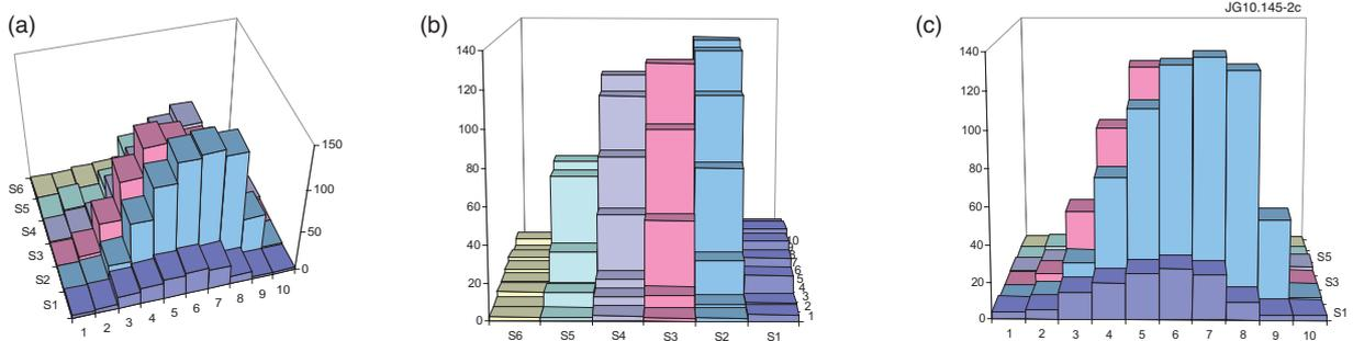
Figure 2: Spatial distribution of the neutron fluence. (a): 2D distribution; (b): radial distribution (machine centre is on the left hand side); (c): toroidal distribution.
