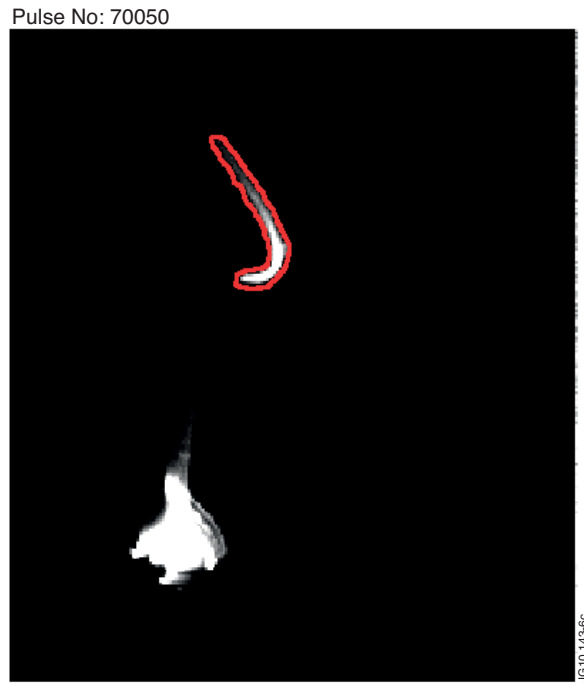
Figure 6: Example of correct detection of a MARFE in a frame of JET fast camera.
