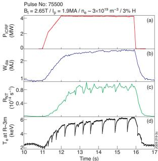
Figure 2: Typical ICRF power levels in ELMy H-mode from (a) the ILA upper half (equipped with in vacuum conjugate-T, (b), antennas A and B (equipped with 3dBs couplers), (c) antennas C and D (equipped with external conjugate T).
