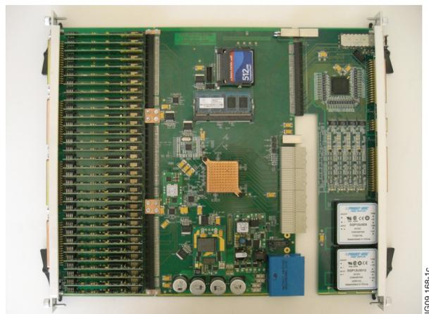
*Figure 1: ATCA-MIMO-ISOL module top view (including the ADC modules carrier board, main controller and Rear Transition Module board).*
