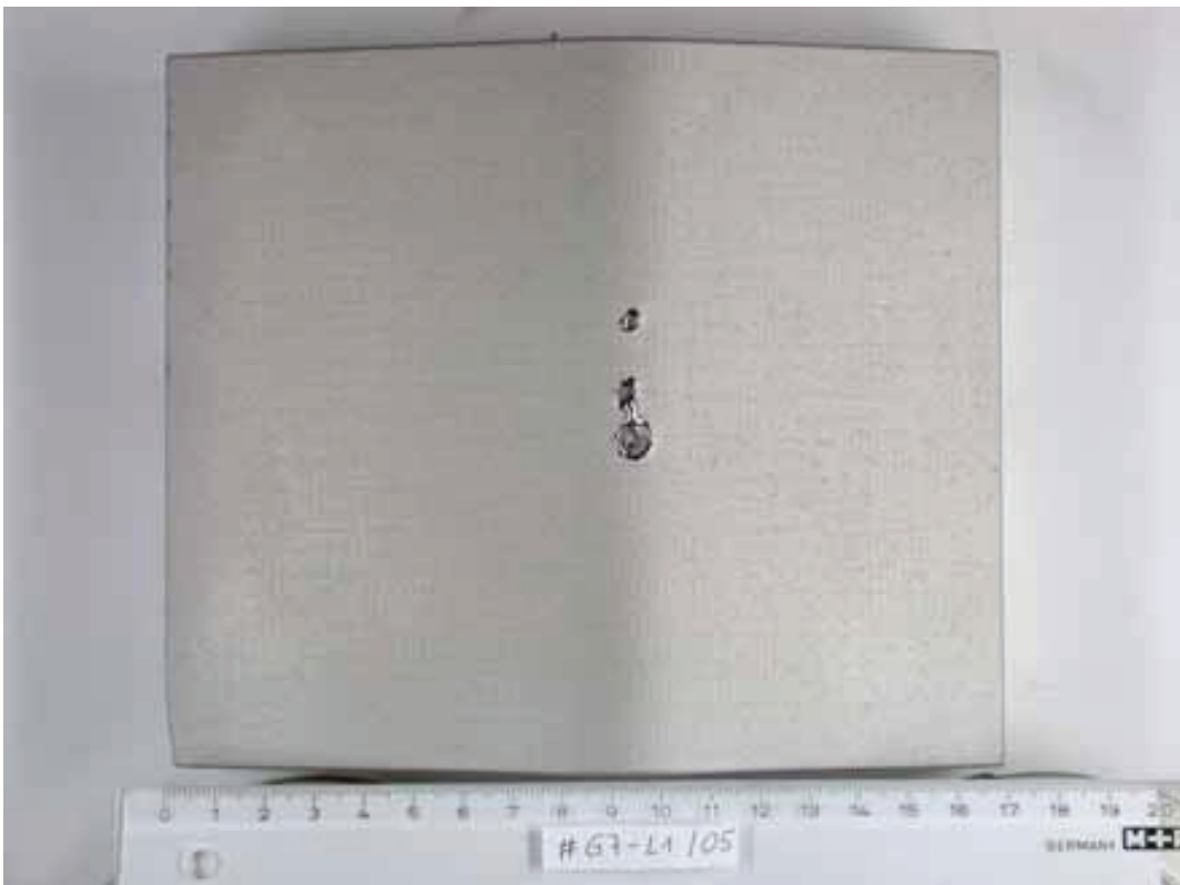
Figure 2: VPS coated large test tile after high heat flux loading in GLADIS for 43 pulses at 16.5\text{MW/m}^2 and a pulse duration of 0.5s. The scale is in cm
