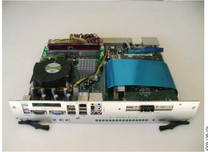
Figure 10: ATCA-CONTROLLER-PCIe board (RTM power supply not shown).
