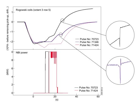
Figure 2: Raw signal of a Rogowskii coil before (Pulse No; 70723) and after (Pulse No's: 71346 and 71424) the 2007 repair which removed plasma and NB drift and step at the disruption.
