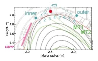
Figure 1: Schematic summarising the layout of the halo current diagnostics in the top of the JET vessel.(1992): one TF pick-up coil behind the centre of the dump plate (oct 3) and two mushroom tiles (MT1 and MT2) shunts.
