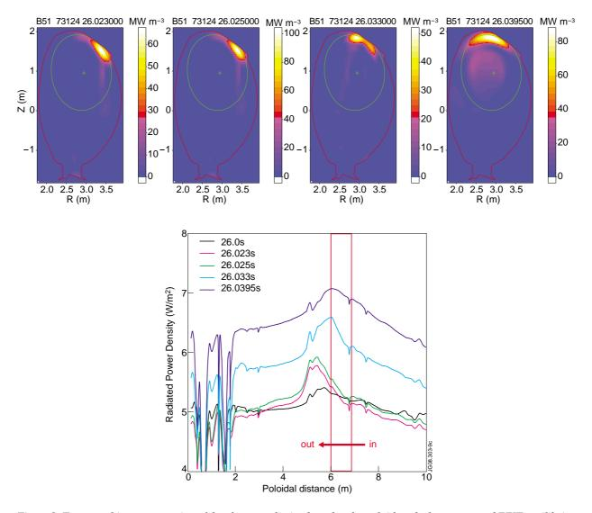
Figure 9: Tomographic reconstruction of the plasma radiation based and overlaid on the last converged EFIT equilibrium during the vertical displacement (a) and (b), at the thermal quench (c) and at the total radiation peak (d) for Pulse No: 73124 above and on the left the radiation poloidal profiles at the same times as the tomographic reconstruction and before the vertical instability was initiated; here the dump plate is between 6.0m (outer) and 6.8m (inner).
