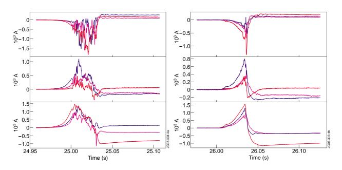
Figure 4: Halo current collected in rows 1, 3 and 5 of the HCS in octants 1, 3 and 7, with the selected set of polarities for two typical pulses.
