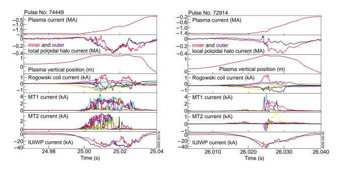
Figure 3: Overview of halo diagnostic observations for two typical ohmic vertical disruptions: (a) low triangularity - Pulse No: 74449 and (b) high triangularity - Pulse No: 72914.
