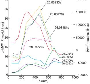
Figure 7: Collected halo current density on the dump plate at octant 3 during the VDE of Pulse No: 73124 (high energy, high triangularity), together with the plasma current and the poloidal halo current seen by the TF pick-up coils at the inner and outer edge of the dump plate at octant 3.
